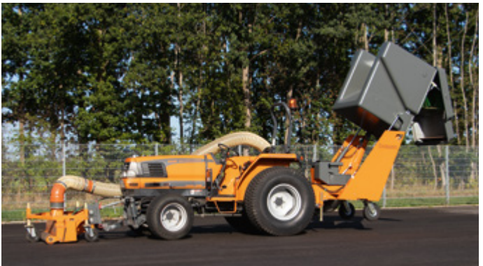
Compact tractor with bema suction sweeper in combination with bema tipping container incl. chaff blower in the rear
