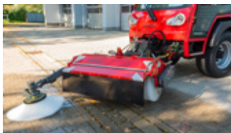
Free sweeping sweeper with protective cover rotary side brushes and water-spraying device
