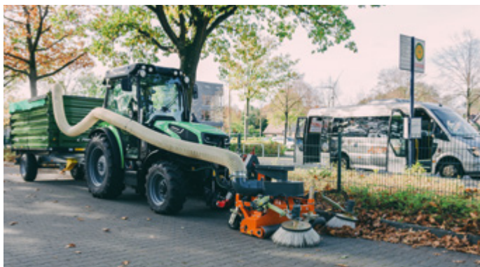
Compact tractor with bema suction sweeper incl. chaff blower and two rotary side brushes in combination with an existing collection trailer (third-party system) in the rear
