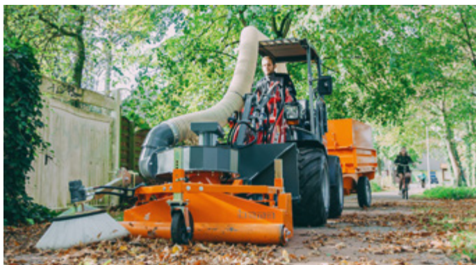
Yard loader with bema suction sweeper incl. chaff blower and one rotary side brush in combination with an existing collection trailer (third-party system) in the rear
