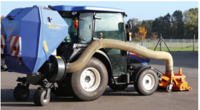
Compact tractor with bema suction sweeper in combination with an existing suction container (third-party system) in the rear
