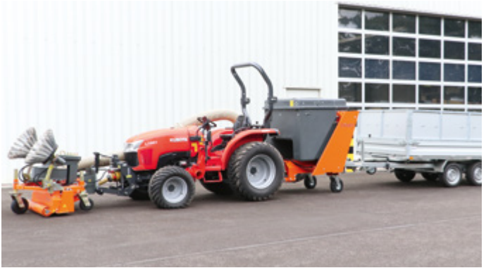
Compact tractor with bema suction sweeper incl. chaff blower and two rotary side brushes in combination with the bema tipping container and another trailer in the rear
