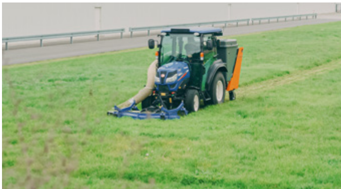
bema tipping container incl. chaff blower combined with an existing mower
