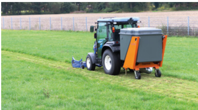
Mowing and collecting the cut grass in a single working step
