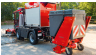
Complete rear unit: Suction sweeper, chaff blower and tipping container
