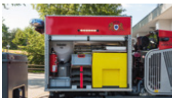
The platform of the narrow-track municipal vehicle accommodates the tank for surfactants and the distributor for the oil binding agent
