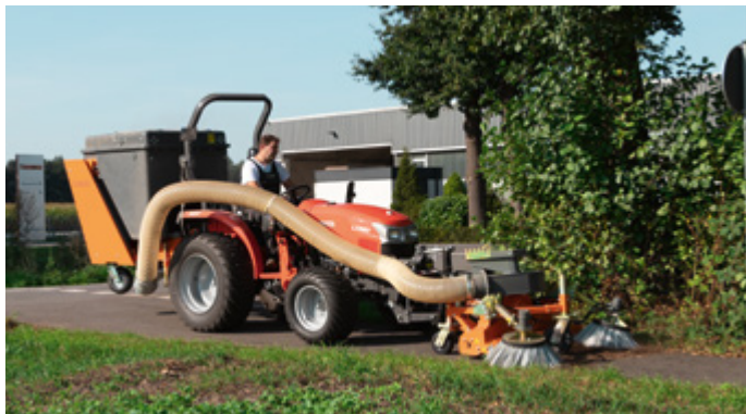
Compact tractor with bema suction sweeper incl. chaff blower and two rotary side brushes in combination with the bema tipping container in the rear
