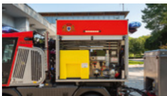
The platform of the narrow-track municipal vehicle accommodates the tank for surfactants and the distributor for the oil binding agent
