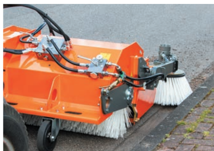
Hydroblock and rotary side brush with bema SideControl
