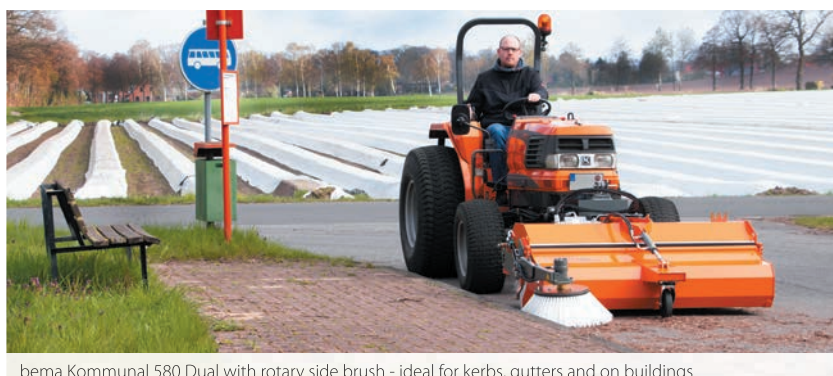
bema Kommunal 580 Dual with rotary side brush - ideal for kerbs, gutters and on buildings
