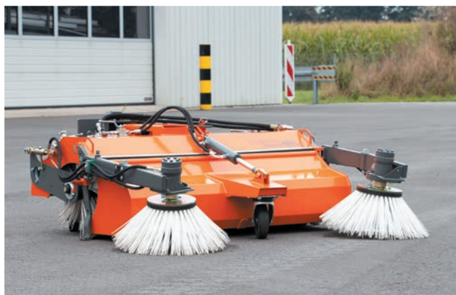
bema Kommunal 450 Dual with two rotary side brushes
